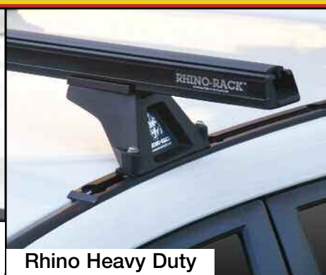
Unique pivoting rear spacer blocks enabling the rear bar to stay parallel to the front bar (Included in Track Kit).
